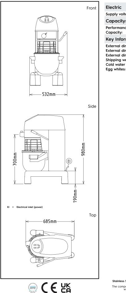
Electric Supply voltage: 200-240 V/1N ph/50/60 Hz Capacity: Performance (up to): 6 kg/Cycle 20 litres Capacity: Key Information: External dimensions, Width: 521 mm 685 mm External dimensions, Depth: 980 mm External dimensions, Height: Shipping weight: 87 kg 6 kg with Spiral hook Cold water paste: 32 with Whisk
